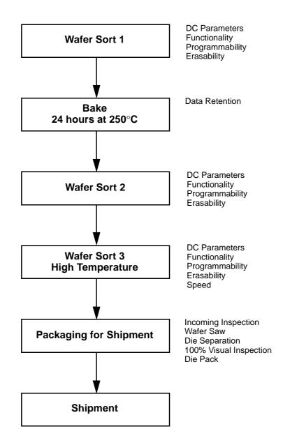
Figure 1. AMD KGD Product Test Flow
